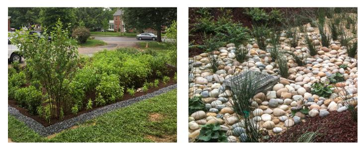
**Green Infrastructure:** *Rain garden and landscaping that work to reduce flooding and pollution caused by stormwater.*
